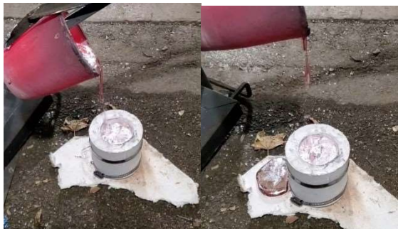
Figures Seven & Eight: Pouring the Molten Aluminum
