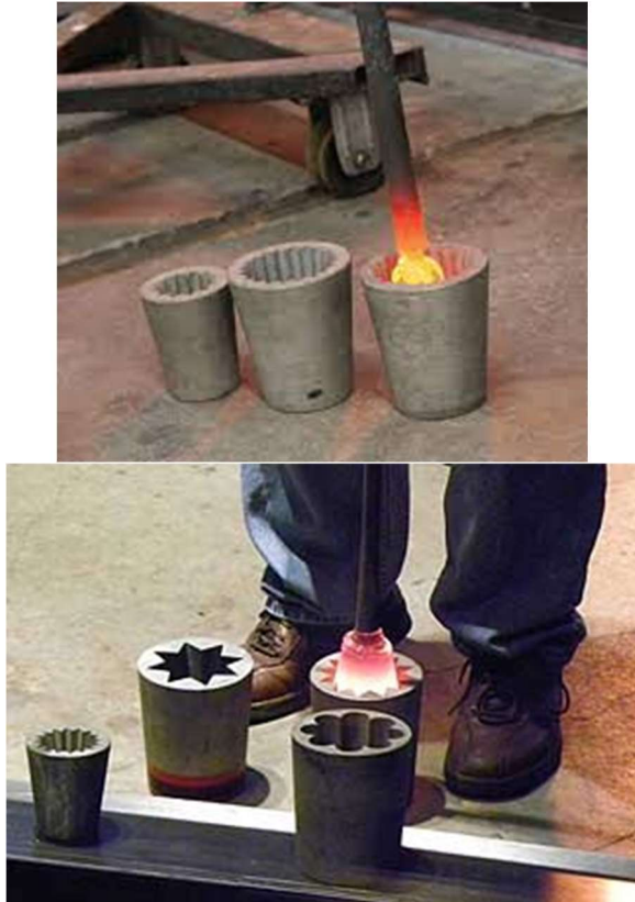
Figures Ten & Eleven: Using an Optic Mold [1] [2]
